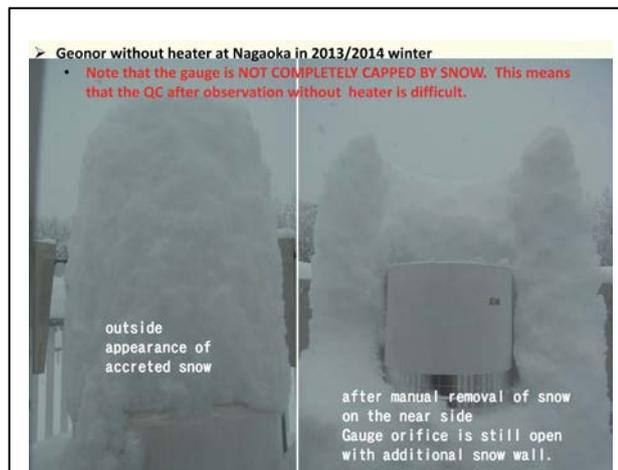
Fig. 4 Snow accumulation on Geonor gauge at 1010 JST on January 11, 2014.
