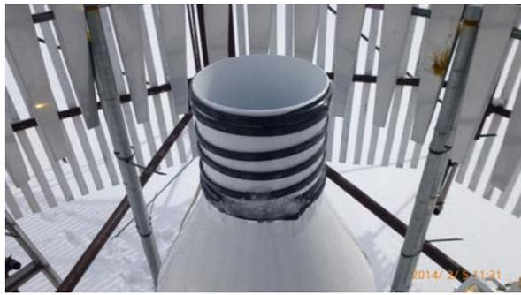
Fig. 3 Close view of the heater and orifice of the gauge.
